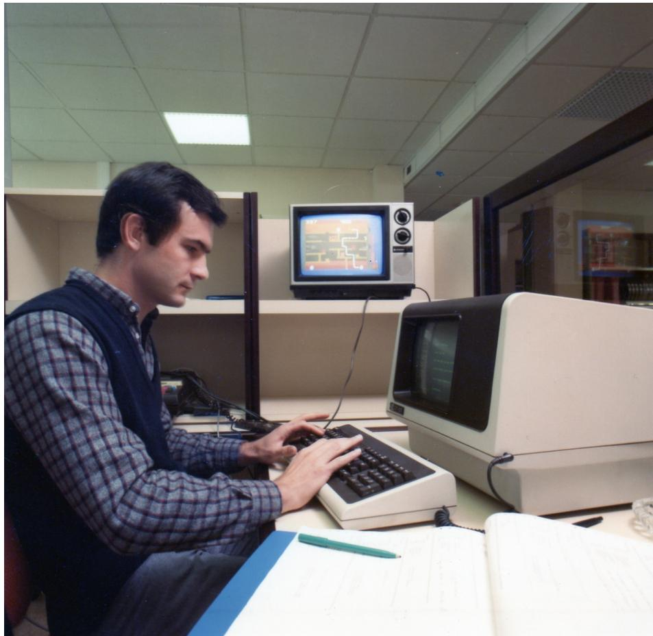
That terminal appears to be a [C. ITOH CIT101 VT-100 clone](#). That terminal sports [two bidirectional serial ports and the ability to bridge between them](#). That seems ideal for this particular use-case.
