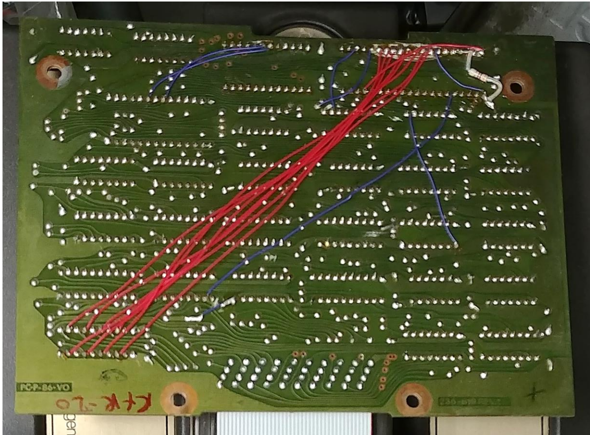
Figure 48 : Joe Jacobs / Dennis Clark Digital Board Solder Side Patches
