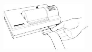
In order to indicate the validity of the seven data lines, another signal must be presented by the host computer to verify that it is placing valid information on them. This strobe signal is accepted on the same trace on the edge connector as the serial input data stream. (NOTE: The complete pinout of this edge connector may be found in the Appendix.)
